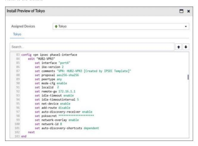
The administrator used the SD-WAN overlay template to prepare an IPsec tunnel configuration for a hub-and-spoke SD-WAN topology. The exhibit shows the FortiManager installation preview for one FortiGate device.
